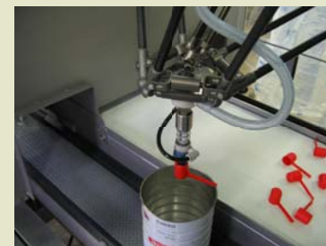
Reliable scoop inserting in can
