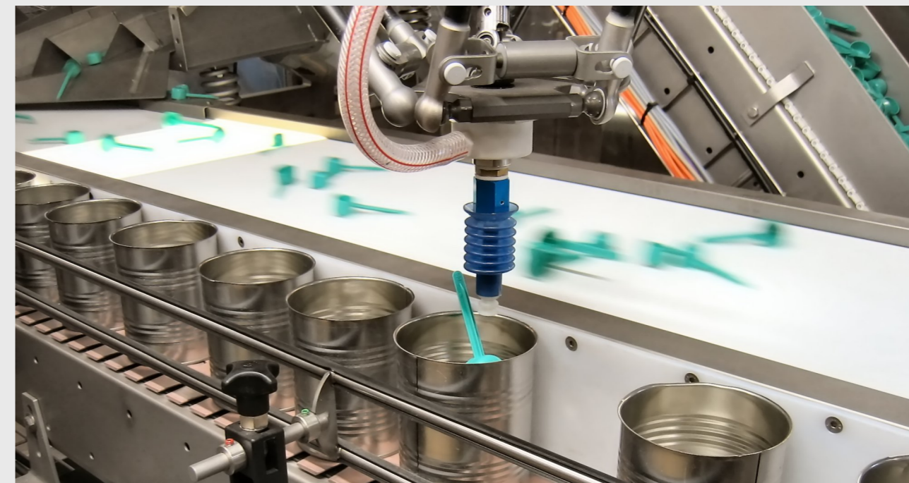
The flexible system handles up to 120 picks/min. per robot with all kinds of packages, scoops etc.
