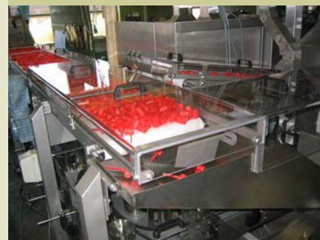
Scoop infeed and scoop return
